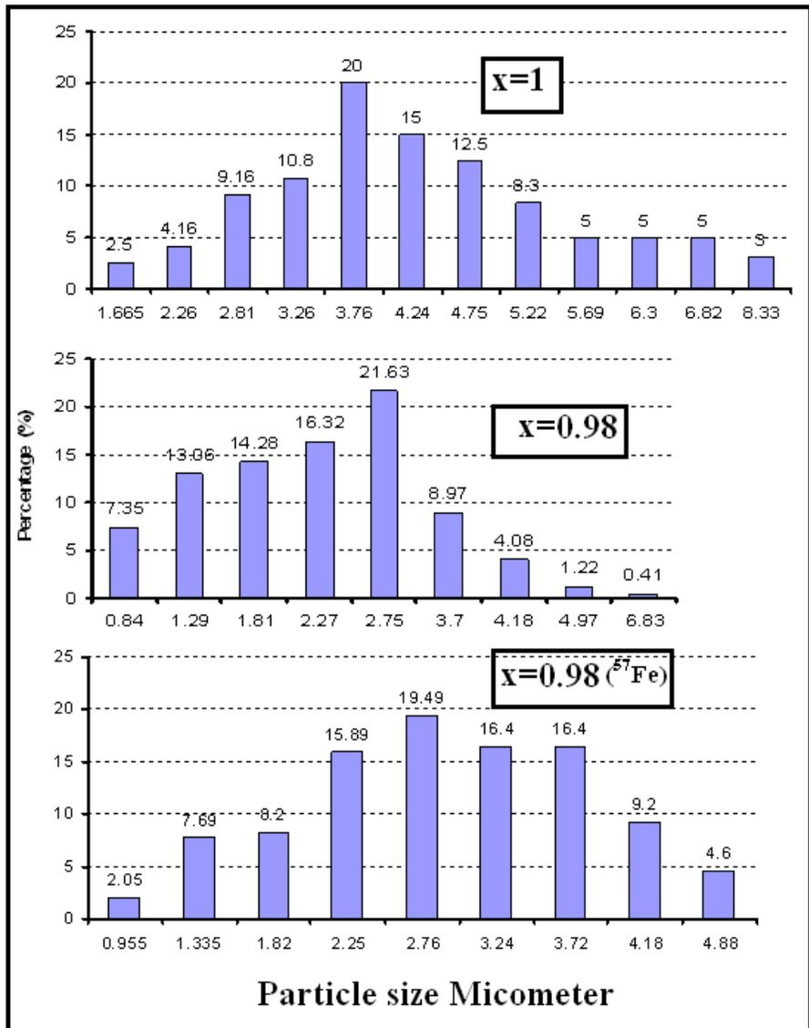
**Fig. 3.1** The particle size distribution of  $\text{Yb}_{0.6}\text{Sr}_{0.4}\text{Mn}_x\text{Fe}_{1-x}\text{O}_3$ .
