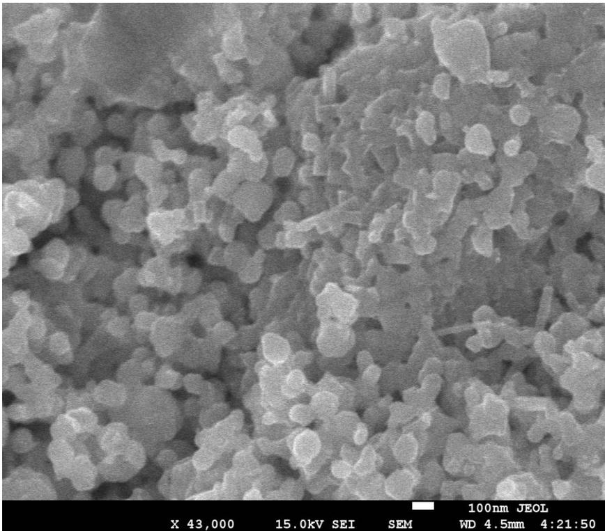
**Fig. 3.4** Microstructure of the  $Yb_{0.9}Sr_{0.1}MnO_3$  composite.
